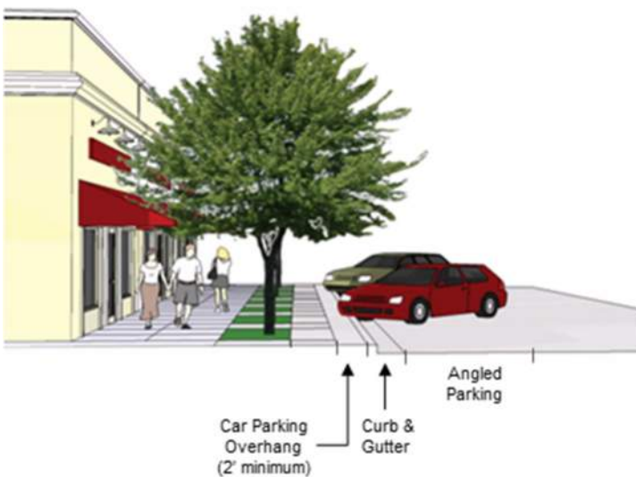
Source: Jacksonville Design Guidelines and Best Practices Handbook (Section 1: Commercial Development) Figure 2.5-2 Angled parking diagram
