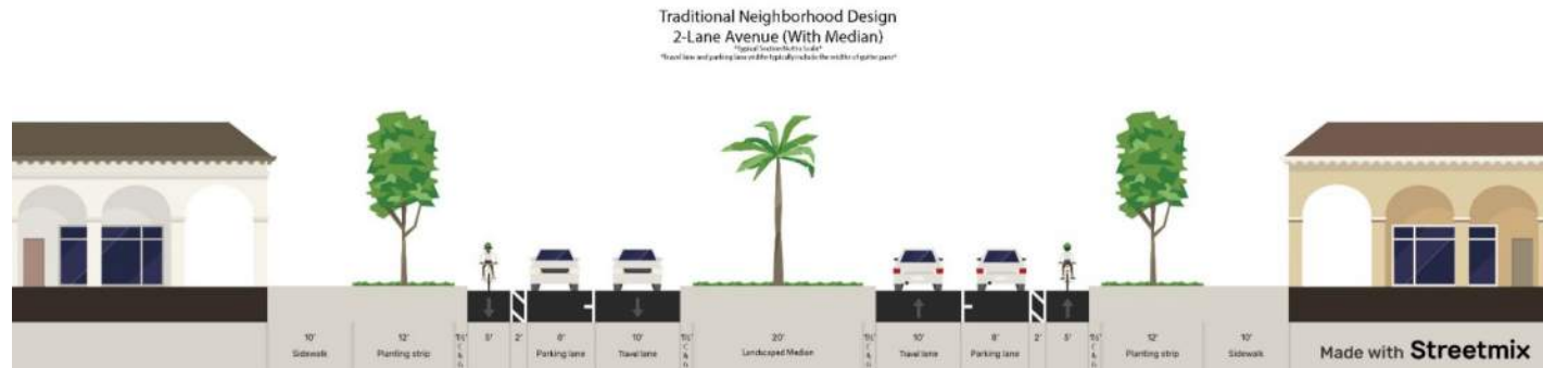
Figure 3.4-4 TND 2-Lane Avenue with Median
