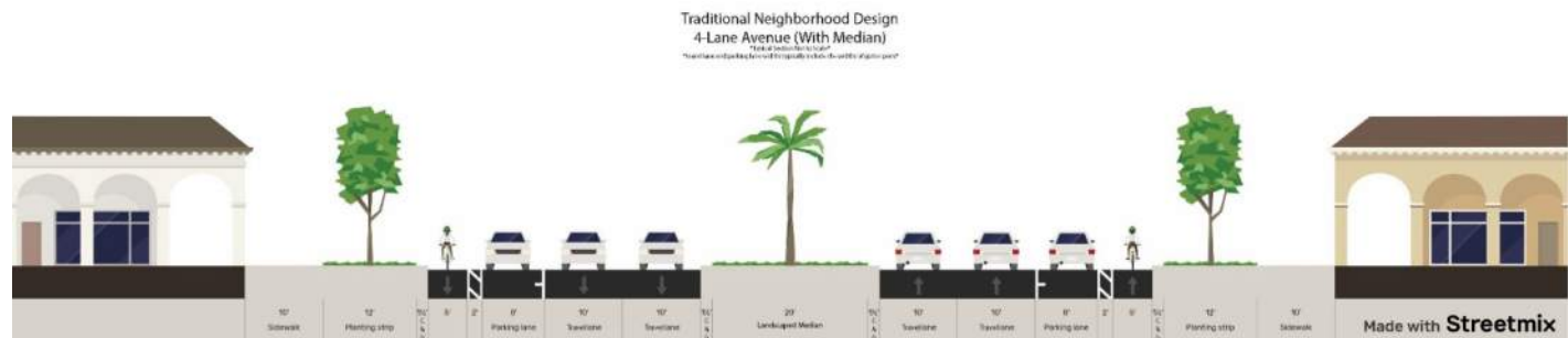
Figure 3.4-6 TND 4-Lane Avenue with Median
