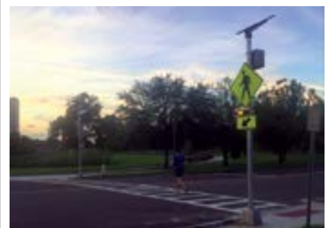
A new RRFB on Pearl Street along the Hogans Creek Greenway in Henry J. Klutho Park
