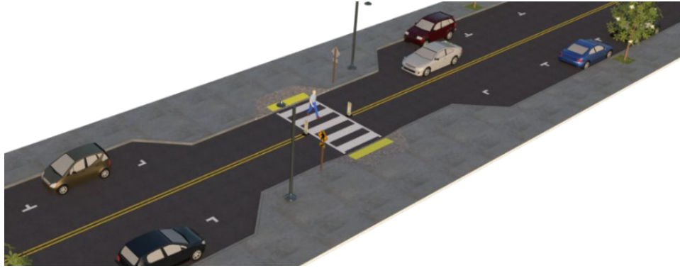
Figure 25. Graphic. Concept demonstrating curb extensions on both sides of crosswalk (VHB, 2018).*
