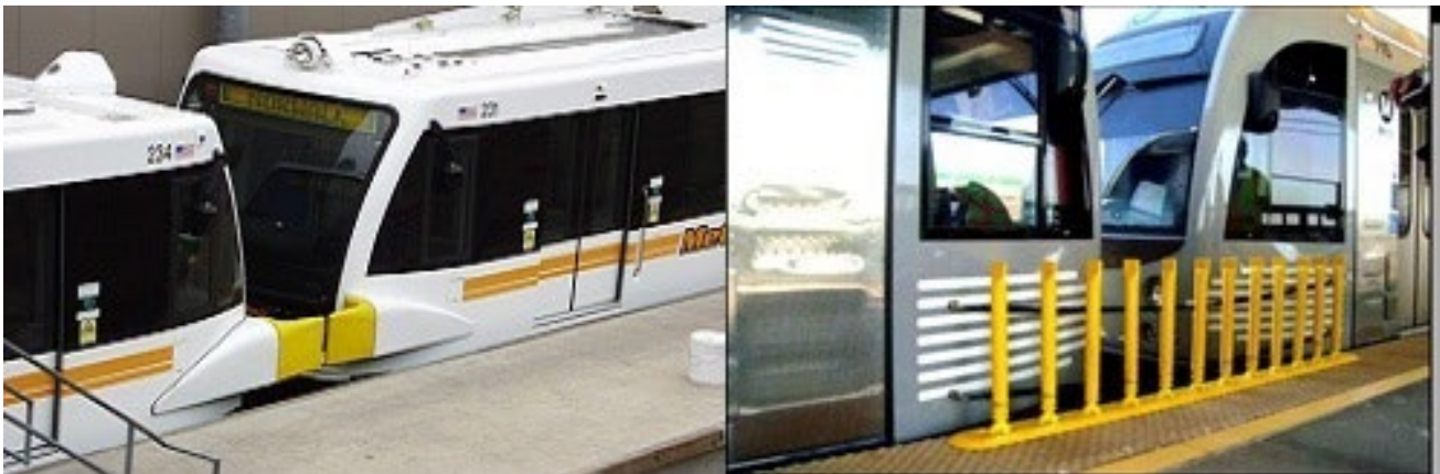
Figure 18. Photograph. Examples of between-car-barriers for light rail (FTA, 2019).
