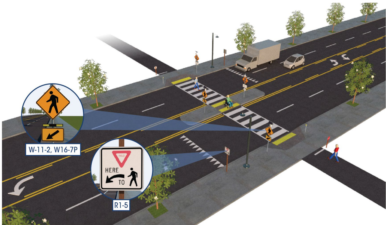
Figure 28. Graphic. RRFB featuring pedestrian refuge island (FHWA, 2018c).
