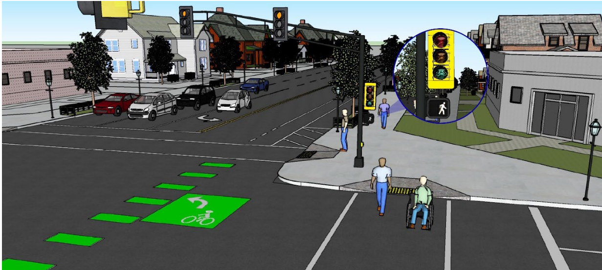
Figure 32. Graphic. Concept demonstrating pedestrian and bicycle signals (VHB, 2021).*
