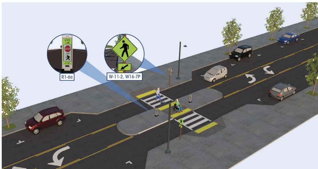
Figure 23. Graphic. Pedestrian refuge island concept featuring pedestrian regulatory and warning signs (FHWA, 2018a).
