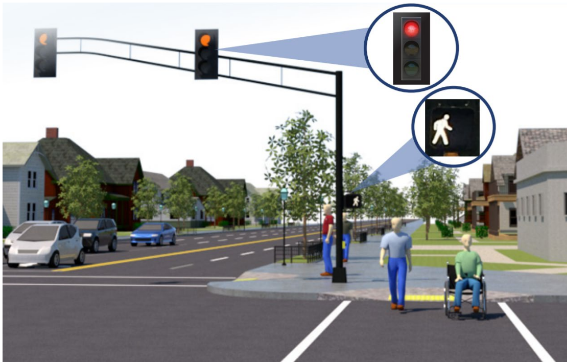
Figure 34. Graphic. Concept demonstrating an all-red signal during the LPI phase (FHWA, 2019).
