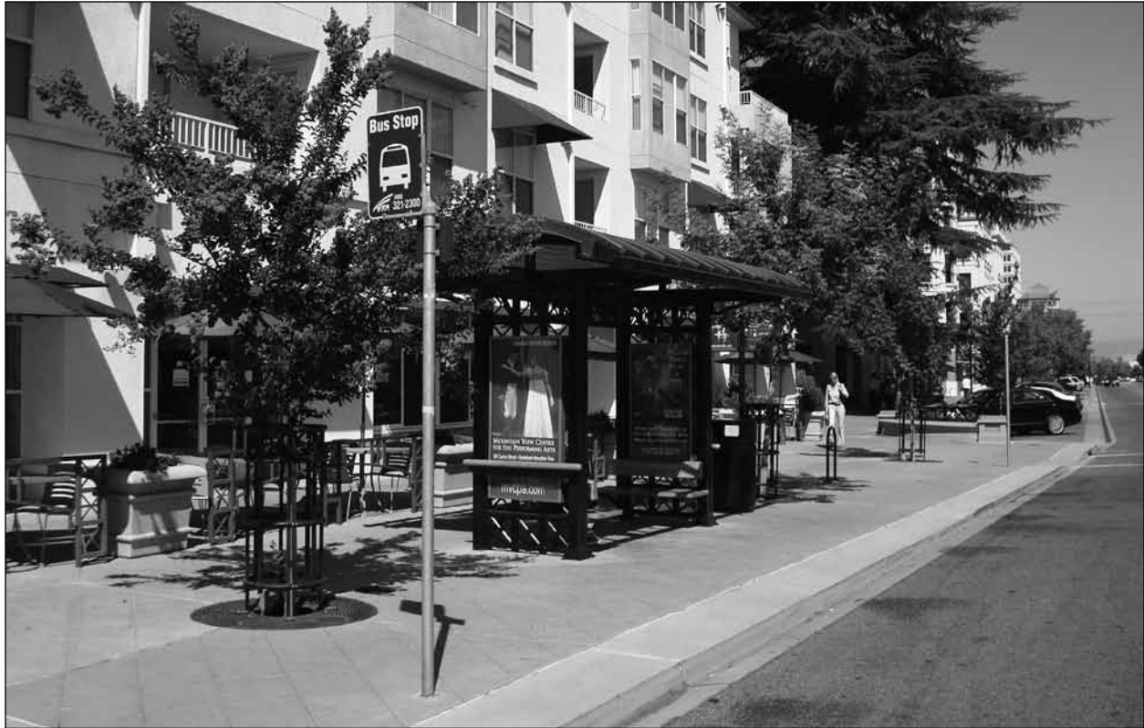
Figure 8.5 Utility poles and other fixtures should not interfere with the pedestrian thoroughway. This example shows a bus shelter and other street furniture properly located in the furnishings zone. Source: Kimley-Horn and Associates, Inc.
