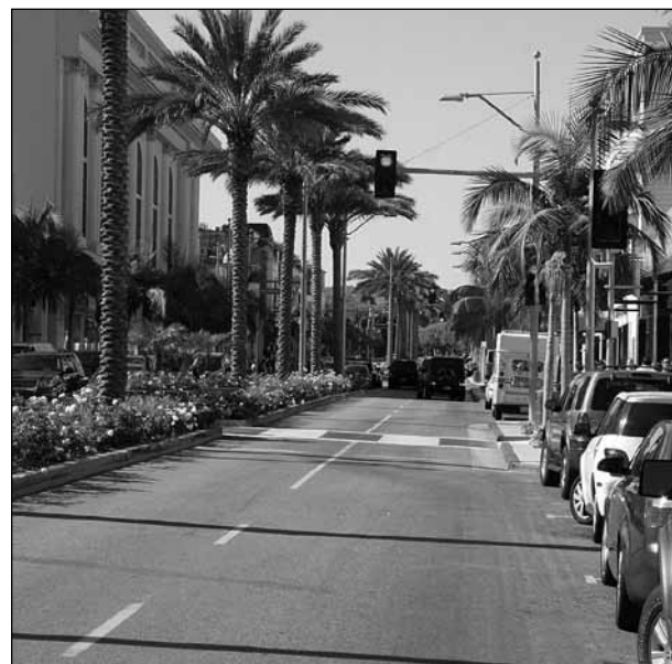
Figure 9.7 Maintain a minimum 18-inch offset between the face of median tree (at maturity) and the face of curb. Source: Dan Burden, walklive.org.
