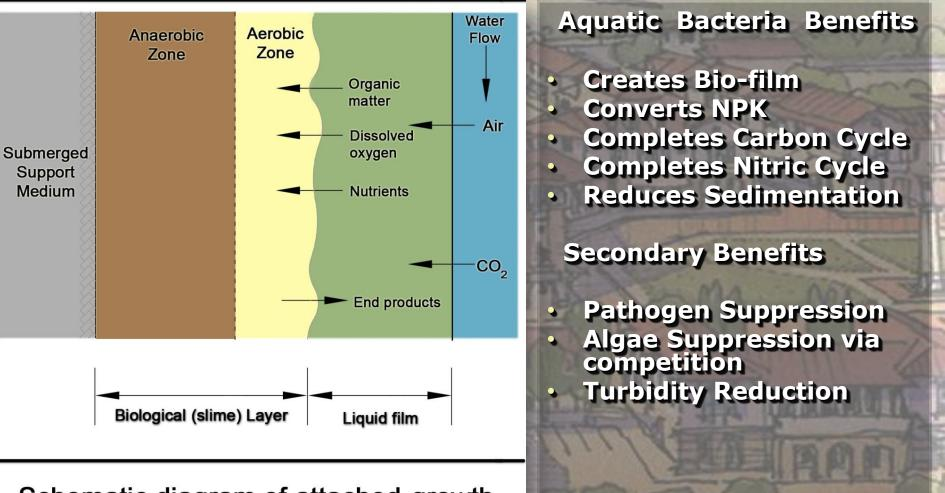
Schematic diagram of attached-growth
