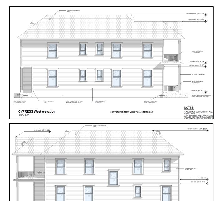
CONCRETE BLOCK STEM WALL WITH PAINTED FINISH (TYP.)
