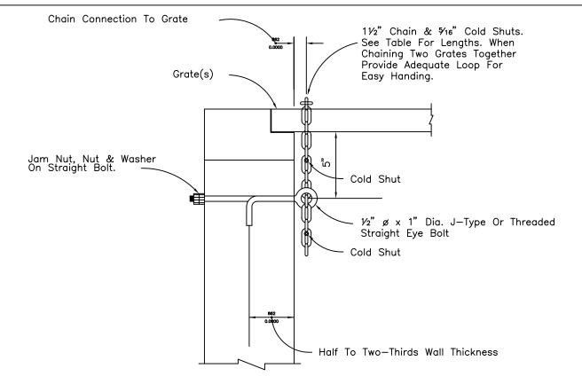
Cost of Galvanized eye bolt and chain to be included in the contract unit price for inlet.
