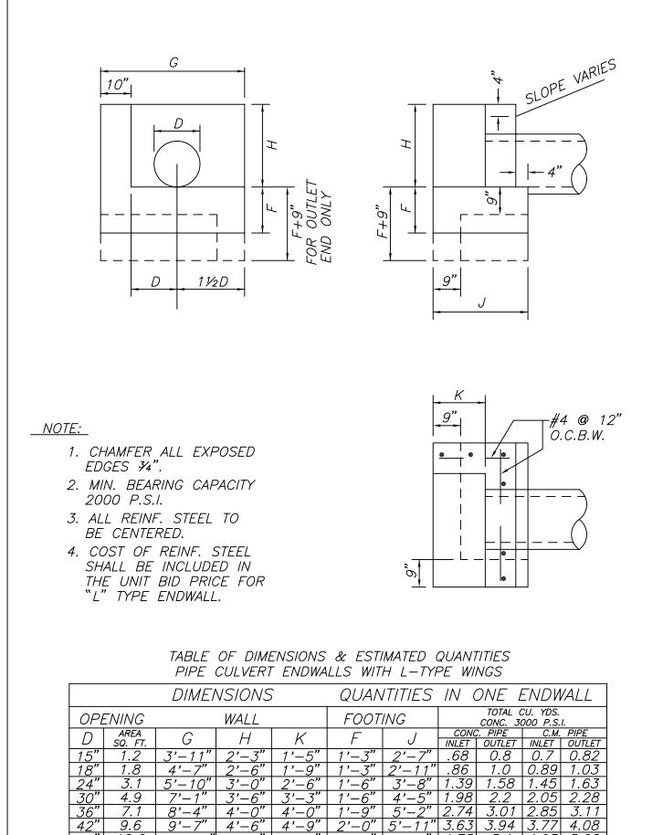
48" 12.6 6'-8" 5.1 4.93 5.28 10' - 1051 '—O' 4.75 CITY OF CONCRETE ENDWALL N.T.S. PLATE D-428 WITH L-TYPE WING JACKSONVILLE DATE DRAWN 2-78 FOR PIPE CULVERTS **STANDARD** REVISED DATE 5-12-94
