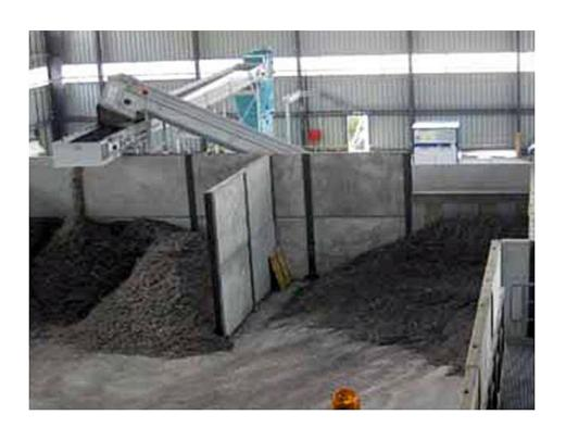
Finished RDF ~ 25 mm Titan's Zlatna Panega Plant in Bulgaria
