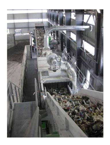
Wind Sifter (Light Fraction Separation) Titan's Zlatna Panega Plant in Bulgaria
