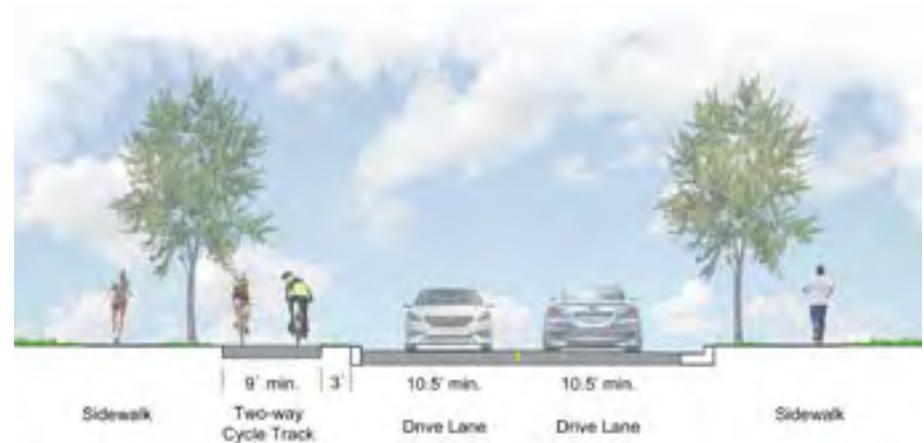
Raised Two-way Cycle Track Typical Section
