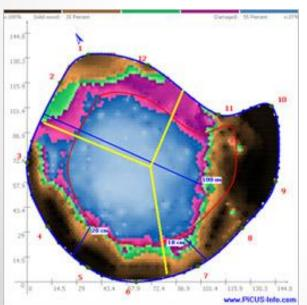
A device that listens to how sound waves move through the trunk/branch. A series of listening devices are attached around the trunk/branch and connected to a computer.
